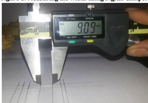
Figure 2: Measuring the width using Digital Calliper
